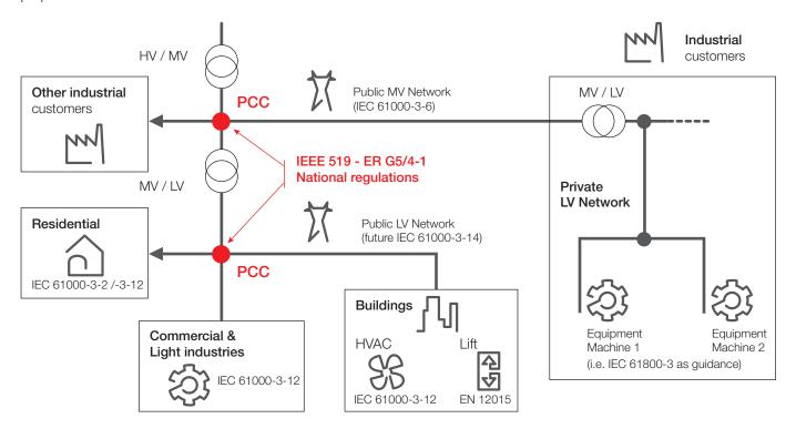
The  $THD_u$  limits are considered at the PCC within the public network (LV or MV) where the different customers are supplied by the Utility. Limits must be applied at the PCC in order to ensure the Utility (often by duty constraints) supplies the different customers with a good quality of power, i.e. with non distorted voltage.
