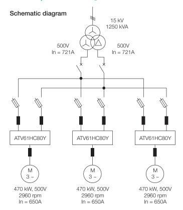
By choosing Altivar frequency converters, the benefits for the customer are that the drives are prepared for 12-pulse connection as standard and no additional equipment has to be ordered. Besides, Schneider Electric offered an "Engineered Drives" solution ready to use with all necessary components within proper cubicles.
