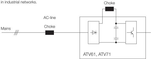
If AC-line or DC-link chokes are not sufficient for a large drive, a multi-pulse arrangement is the next step to consider.
