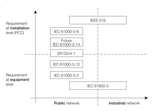
It should be noted that too stringent harmonic emission limits could become very expensive. That's why a careful application of standards should be performed. The following diagram is proposed for clarification.
