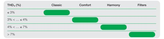
When contractual emission limits are to be met at the installation level, a harmonic study is required. The possible filter may be of different technologies:
