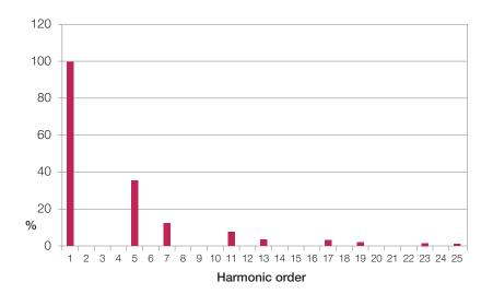
The current distortion can be reduced by implementation of harmonic mitigation. As an example, the improvement provided by a 12-pulse arrangement is presented on the opposite figure. THD $_{\rm i}$  is reduced from 40 to 11%
