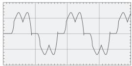
Equipment comprising power electronics circuits are typical non-linear loads. Such loads are increasingly frequent in all industrial, commercial and residential installations and their percentage in overall electrical consumption is growing steadily.
