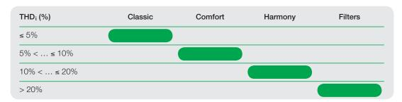
• According to the percentage of total harmonic voltage distortion THD<sub>u</sub> measured at the transformer secondary, at **maximum load and with no capacitor connected:**
